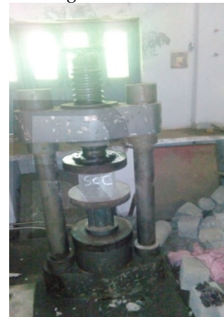
Fig 1 Compressive strength test
